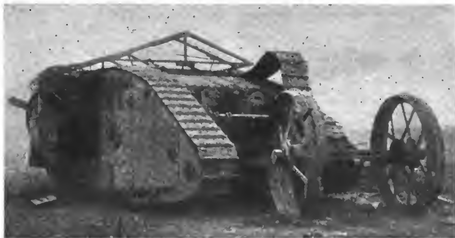
The above illustration is the first authentic picture of one of the caterpillar armored tractors used by the British Army on the Somme front in France. This machine has been injured by shell fire, or otherwise, as one of the elliptical belts which provide traction is torn out of position as shown at the right. Powerful gears revolve the belts and the weight of the machine is carried on rollers which are set close together on the ground side. The large wheels shown in the rear do the steering and support the weight of the tractor when crossing a shell crater or trench, thus greatly increasing its mobile length. Each machine is fitted with three or four machine guns and can fire 2000 bullets a minute, according to reports from the scene of operations.
